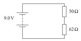
(a) Calculate the power dissipated in the  $62\,\Omega$  resistor.
