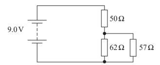
Calculate the total resistance of the circuit.
