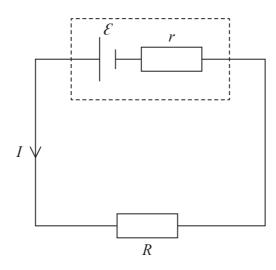
A cell has electromotive force  $\mathcal{E}$  and internal resistance r. It supplies a current I to an external circuit with resistance R.
